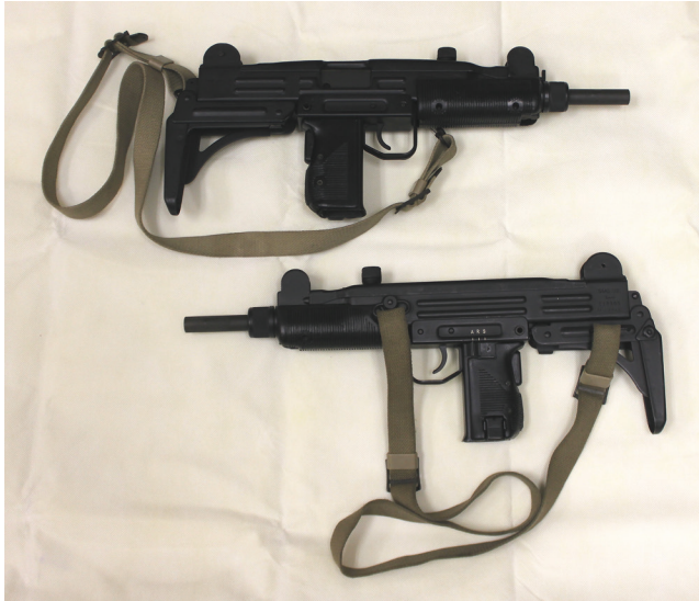
Figure 4.28 The Uzi submachine gun. The depicted examples were manufactured as sub-machine guns by Israeli Military Industries in Israel and are so marked on the left side of the receiver as Uzi SMG. The English-marked selector switch is above the trigger, depicted in the lower example. Hebrew-marked selectors are also encountered. (Image from author's collection.)
